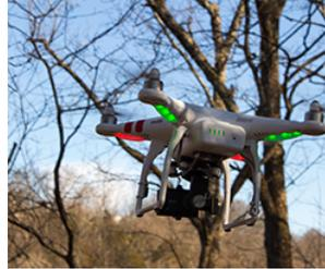
For aerial photos and/or video, HMB purchased a DJI Phantom 2 drone in August 2014. The drone is capable of flying at over 3,000 feet and can record up to 25 minutes of continuous video. HMB currently has two batteries for it, enabling it to record up to 50 minutes in one session. A GoPro Hero 3+ camera is currently attached to the drone
